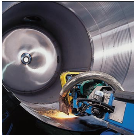
Our inside grinding machine for bodies, dished ends and nozzles works entirely automatically. Perfectly ground steel surfaces form the ideal base for the glass-lining
