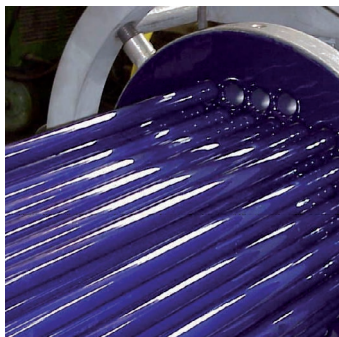
Glass lined U-tube heat exchanger during assembly
