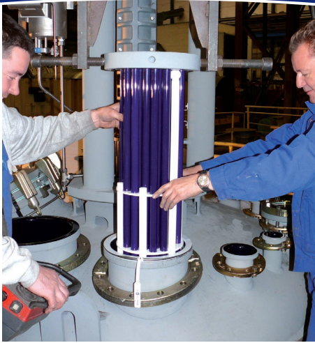
Using a WTU Compact Heat Exchanger as a PowerBaffle (see page 7 for details)
