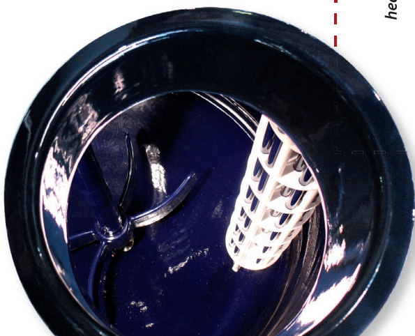
PowerBaffle inside a reactor
