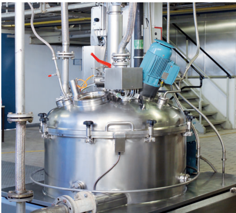
Scraper centrifuge VBC 1000
