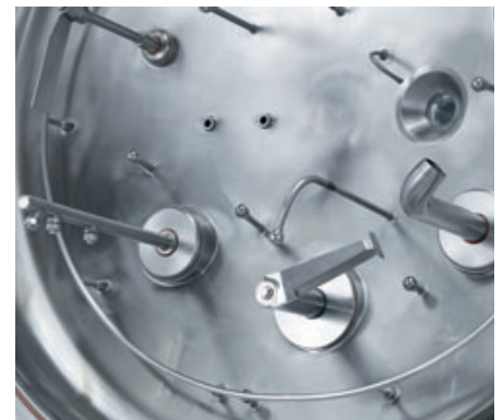
Vertical top discharge centrifuge feed pipe and wash pipe, loosening scraper
