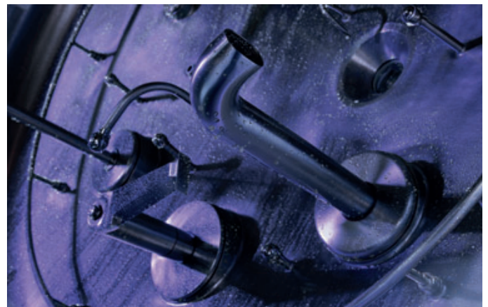
After the CIP program: in UV light no more riboflavin residue is visible
