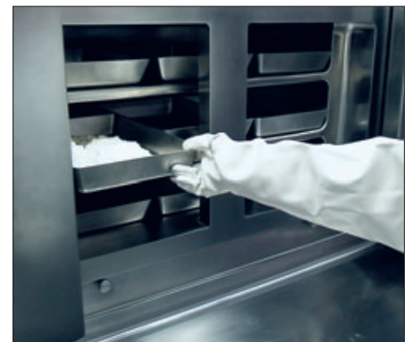
Charging of vacuum tray dryer
