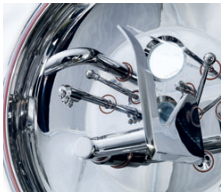
Scraper knife over the entire basket height, feed pipe and wash pipe
