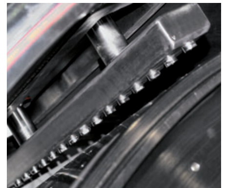
Residual heel removal (single row design)
