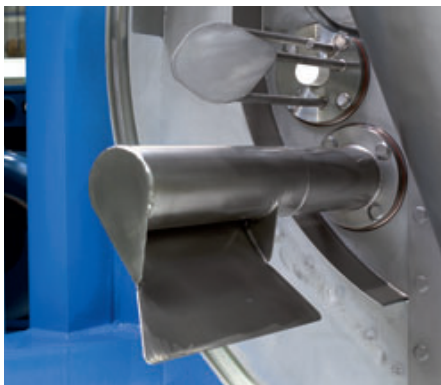
Feed pipe with deflector
