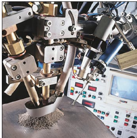
Our submerged-arc automatic welding machine does material-friendly welding based on minimal heat effect for up to 100 m of weld seams per unit
