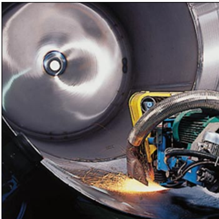
Our internal grinding machine for bodies, dis-hed ends and nozzles works entirely automatically. Perfectly ground steel surfaces form the ideal substrate for the glass-lining
