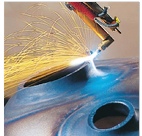
Computer-controlled flame-cutting robots guarantee high-precision synchronous cutting resulting in precise fitting accuracy of neck and nozzles
